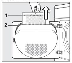
Open the door and pull the fluff filter (1) out of the door as illustrated.
